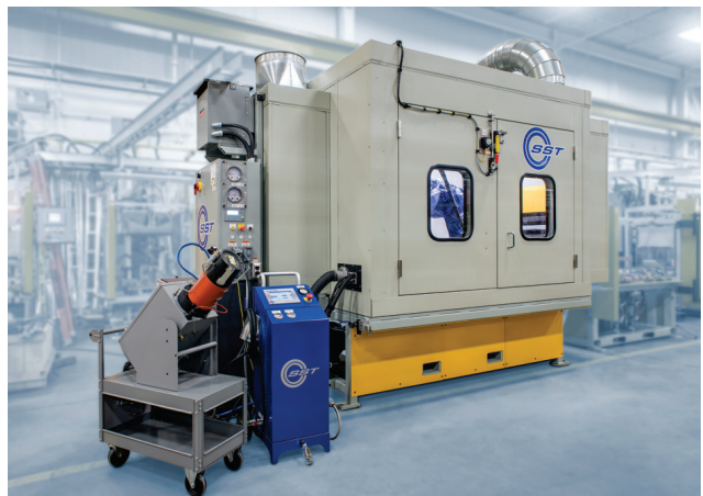
Fig. 3 — Commercial SST cold spray system. Courtesy of CenterLine Windsor Ltd.
